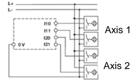
Axis 1 with one incremental encoder to:
