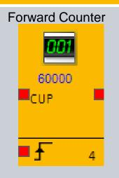
When the status at the input has changed from "0" to "1" a preset number of times, the output on the event counter will switch to "1".
