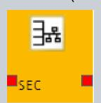
The safe Ethernet connection SEC (Safe Ethernet Connection) enables a point-to-point connection of 48 virtual inputs and 48 virtual outputs between a PNOZmulti base unit and a PSS 4000 device. The inputs and outputs are safety-related.
