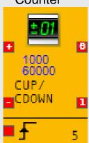
When the status at input 1 changes from "0" to "1", the counter is incremented by one; when the status at input 2 changes from "0" to "1", the counter is decremented by one. The output on the event counter switches to "1" when the specified value has been reached.
